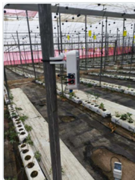
Datalogger enclosure positioned on the stand.
